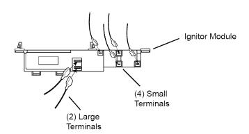
Important: Be sure to attach wires correctly to terminals.
